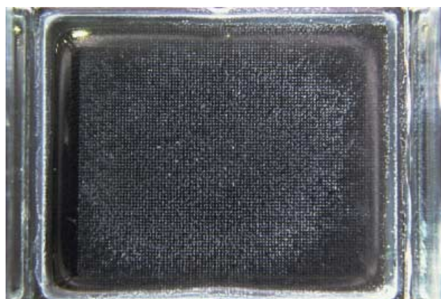
Figure 1. Microarray of ten thousand (100×100) hepatocyte heterospheroids prepared on 100 μm diameter circular glass domains with 100 μm spacing on 20×20 mm glass substrate coated with α-lactosyl-PEG/PLA.
